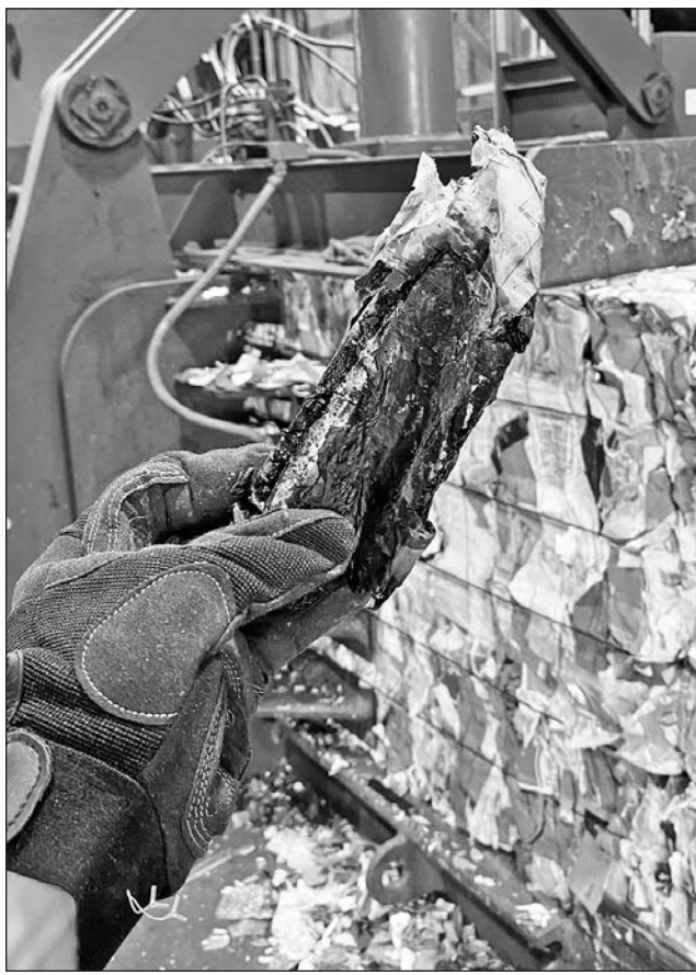
OUTAGAMIE COUNTY RECYCLING AND SOLID WASTE Brodhead Independent-Register A punctured or bent lithium-ion battery can produce enough heat to melt or ignite materials near the battery, even if the battery itself does not ignite.
